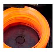
Wire rod coiling Wire rod of up to 10 mm is coiled on a laying a head. Rod in larger diameters is coiled in garrett coilers.
