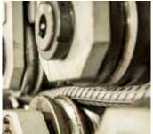
Straightening Rebar coils are straightened before cutting to lengths to remove tension in the material.
