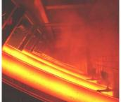
Billet feedstock Our rolling mill uses billet feedstock produced at the SMACC melting shop.
